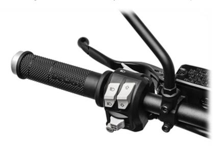
hydraulically operated brake pumps and clutch, making the controls modern yet faithful the classic Scrambler to stvle. Brake and clutch levers are adjustable. The painted die black aluminium footrest plates (grey on the Scrambler 1100 Special) support the gear shift and rear brake levers, both made of forged aluminium.
