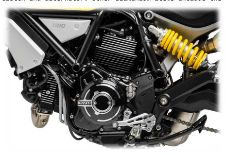
Excellent pulling power is also put within everyone's reach by the 16° valve overlap angle. Thanks to these solutions the Ducati Scrambler L-twin puts out a maximum power of 86 hp at 7,500 rpm and a maximum torque of 88.4 Nm at 4,750 rpm, with smooth delivery across the rev range. The gearbox is a 6-speed unit while the clutch is the wet multiplate type with hydraulic control. The clutch also has a servo-assisted slipper function that limits rear wheel destabilisation during down-shifting.
