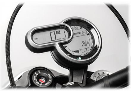
and the selected Traction Control level. Further info includes Trip 1, Trip 2, miles remaining and air temperature, plus grip heater operation (available on the Scrambler 1100 as an accessory). The second, oval element, instead, has a speedo, a kickstand warning light and information from the Ducati Multimedia System, available as an accessory when the Bluetooth module is fitted.
