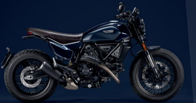
L-Twin, Desmodromic distribution, 2 valves per cylinder, air cooled
